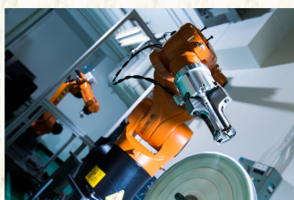
手錶外殼拋光 Watch case grinding and polishing
